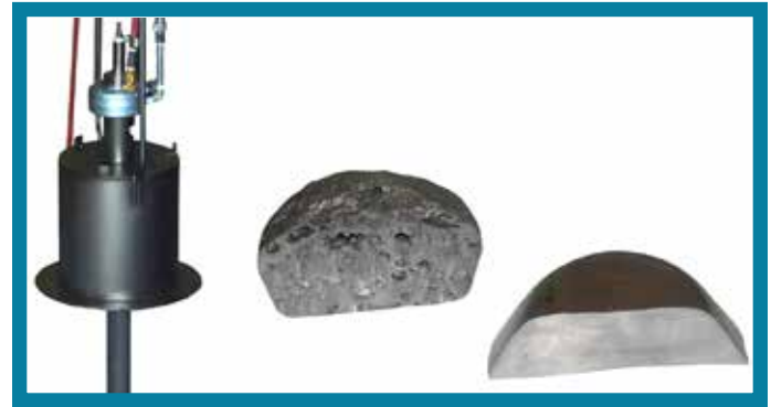
Rotary degasser and samples of clean metal vs bad metal
