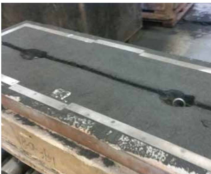
After core is filled, end of vent are shown where the gases are exiting.
